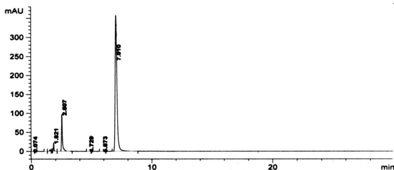
Figure 5: Chromatogram of peroxide degraded sample of Rupatadine Fumarate
