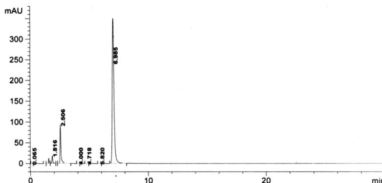
**Figure 3: Chromatogram of acid degraded sample of Rupatadine Fumarate**
