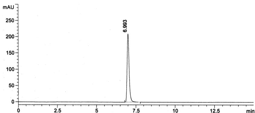
Figure 2: Separation on Spherisorb CN (Cyano), 250 x 4.6mm, 5µ (pH 4.4).
