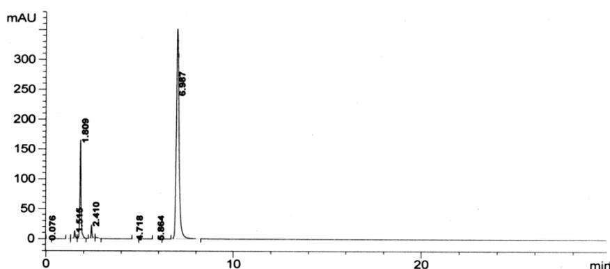
Figure 4: Chromatogram of alkali degraded sample of Rupatadine Fumarate
